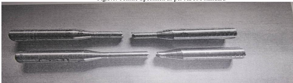
Fig 3.2. Tensile test specimen after test
