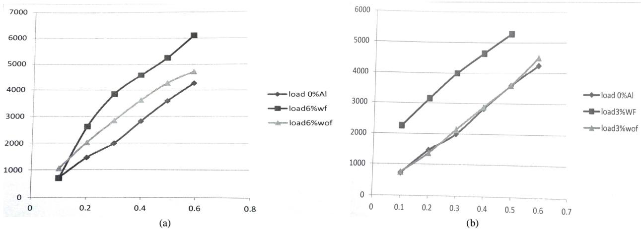
Fig. 4.2: Percentage Elongation as a function of load (Composite with 3wt. % and 6wt. % ZrO<sub>2</sub>)
