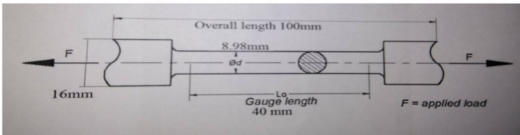
Fig.3.1. Tensile Specimen as per ASTM standard
